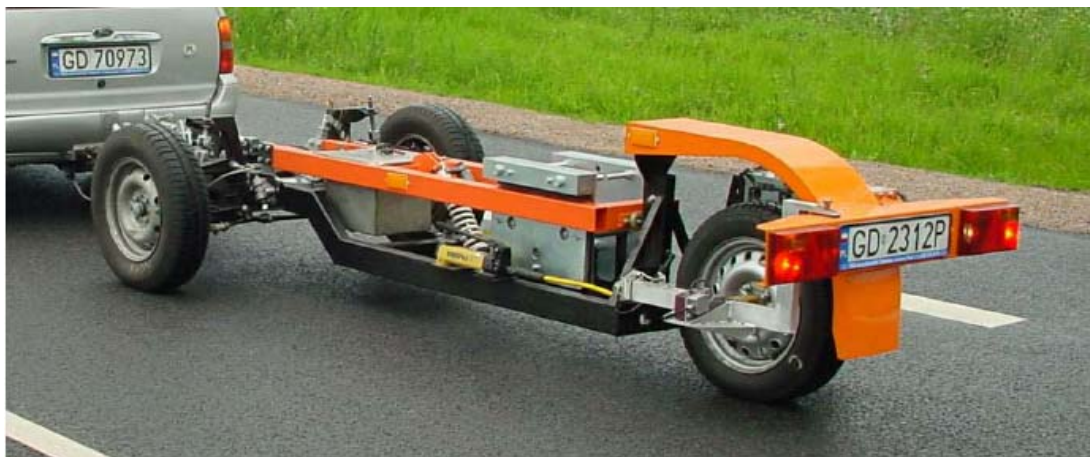
Figure 4-2: Rolling resistance trailer of TU Gdansk, which is also used by VTI
