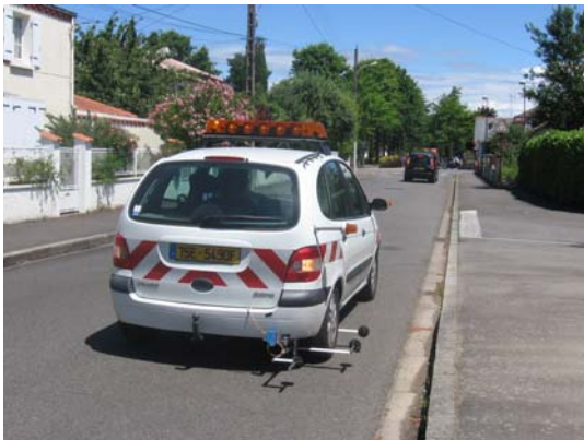
Figure 5-3: Examples of CPX test vehicle (left) and trailer (right)
