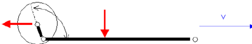
Figure 4-4: Principle of operation of the TUG rolling resistance trailer [18]
