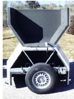
Figure 5-3: Examples of CPX test vehicle (left) and trailer (right)
